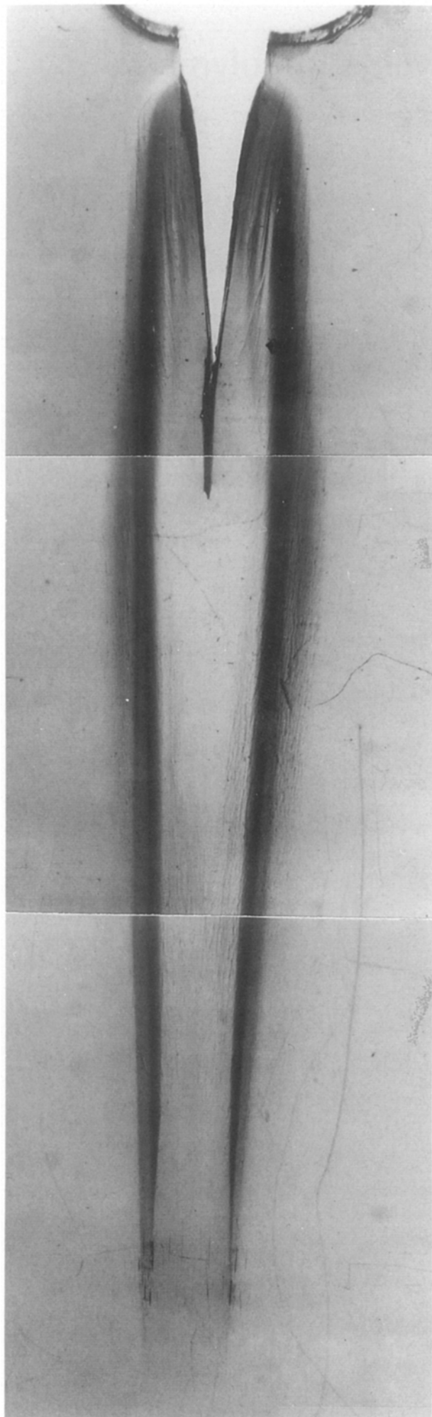
← Figure 1 Optical micrograph of the damage zone produced in a PC-PET sample having the initial dimensions described in the experimental section (approach I).
