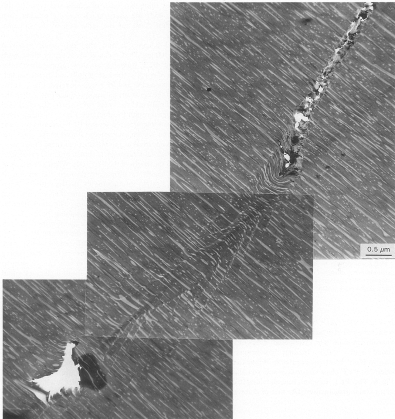
Figure 10 Area in bulk tested PC-PET where the crack stopped when a relatively ductile failure was produced (approach I). The crack integrity was maintained with epoxy for microtomy.
